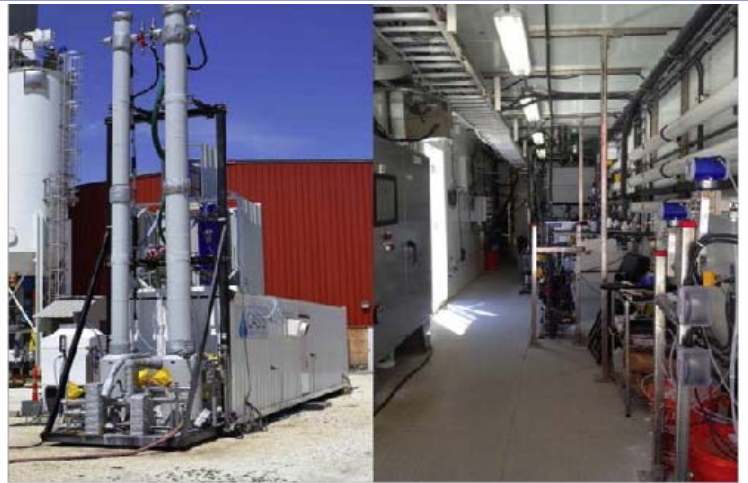
Fig. 4: Novel FO Membrane Brine Concentrator system developed by Oasis Water (From [14]).
