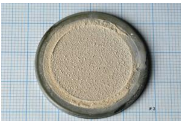
METAL-DOPED SILICA MEMBRANE ON A STAINLESS STEEL SUPPORT, AFTER OPERATING FOR 1100 H IN POWER STATION FLUE GAS. DEPOSITION OF DUST AND PARTICLES IS EVIDENT ON THE MEMBRANE SURFACE.
