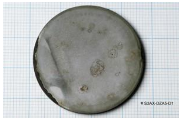
THE SAME MEMBRANE AS AT LEFT, AFTER CLEANING TO REMOVE SURFACE DEPOSITS. THE PARTIAL CORROSION OF THE SUBSTRATE CAN BE SEEN.
