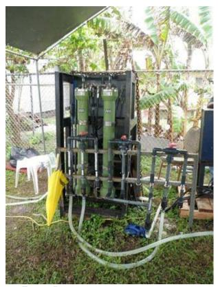
FIG. 2: PORTABLE DESALINATION IN THE MARSHALL ISLANDS (SOURCE PACIFIC ISLANDS APPLIED GEO-SCIENCE COMMISSION)
