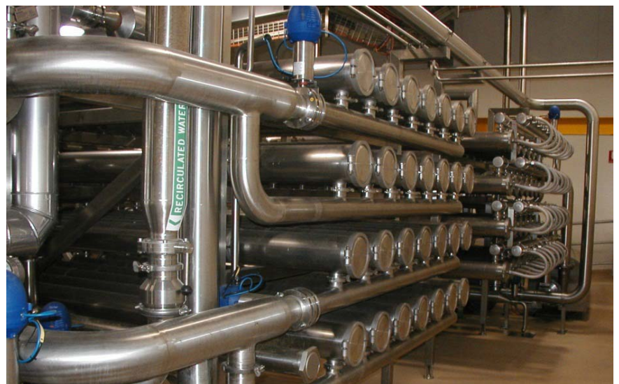
A typical milk UF system (Courtesy Environment Products International Limited, Auckland)
