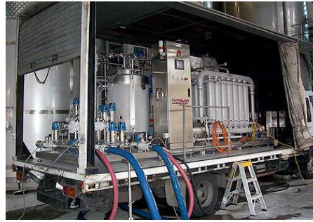
A truck mounted cross flow filtration unit for wine processing (Courtesy Vintech Pacific Ltd).
