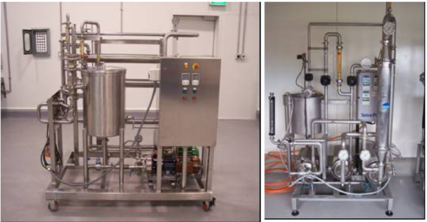
Figure 1. Pilot scale filtration equipment at CSIRO including a membrane filtration pilot plant flexible to perform pilot studies on the full range of membrane filtration technologies (microfiltration, ultrafiltration, nanofiltration and reverse osmosis) under a wide range of operating conditions and a ceramic microfiltration pilot plant.
